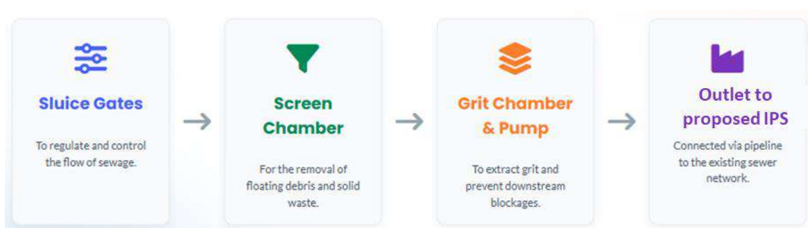
Figure 6-1: Flow arrangement of proposed I & D Structure
